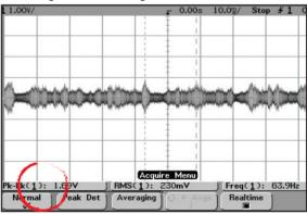
Shaft voltage with carbon fiber grounding ring
